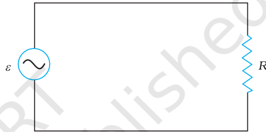
FIGURE 7.1 AC voltage applied to a resistor.
